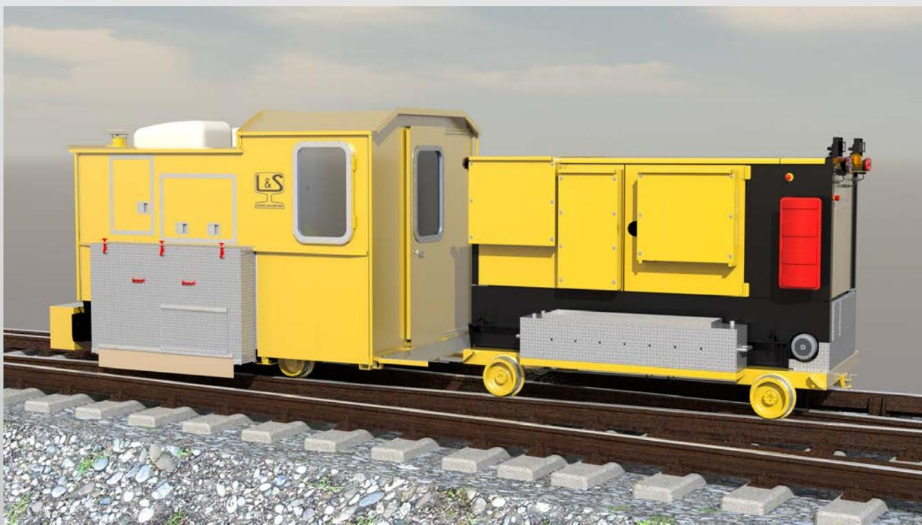
The LRGM 1-6/ AM65 C is a turnout grinding machine with a **closed working platform (cabin)** for the machining of the rail head. It composes except the grinding unit also a generator so that no power cables has to be installed along the working site.
